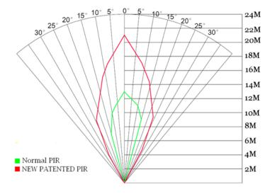
The PIR detection angle ( $\alpha$ ) is just smaller than the field of view (FOV) angle ( $\beta$ ). The advantage of this design is to reduce empty picture rate and capture most, if not all, motions.
